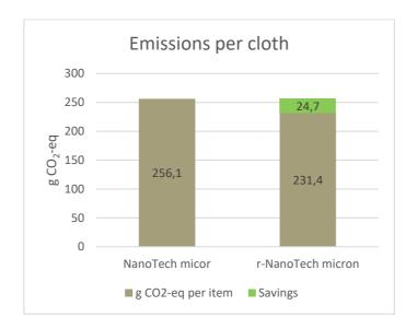
The results show that the production of the basic material has by far the largest share of emissions. This is followed by the dyeing process, end of life treatment, and fabric production. Emissions from converting, packaging production and transportation activities are negligible low.
